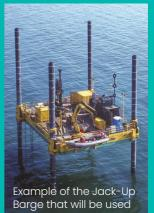
Beginning in mid-July, a Jack-Up Barge will be installed off Fraisthorpe Beach to take various core samples of the seabed and subsurface. The geotechnical surveys will provide information about the physical condition of the seabed. This data will feed into the design and construction of the landfall site for the marine cable.
