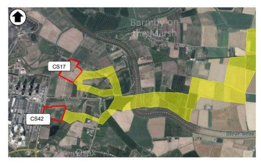
Figure 3 - Preferred route corridor from Asselby to the converter locations. Note site CS42 was selected as the preferred location.
